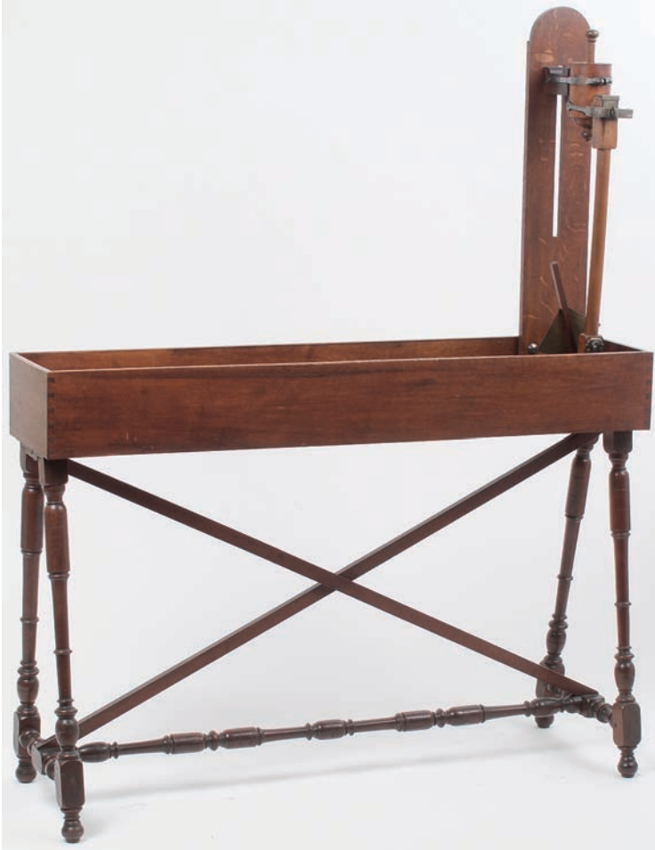
Fig. 2 's Gravesande's mercury fountain. The small reservoir at the top is filled with mercury, which descends through the rod and is projected diagonally into the through.
